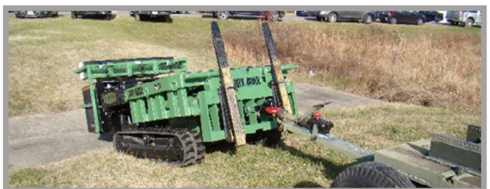
Hitch Receiver for Towing in Unimproved Terrain
