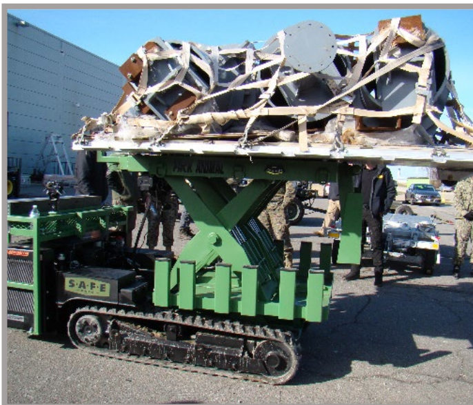
Scissor Deck Lifting Ability of 10,000+ lbs to 65"
