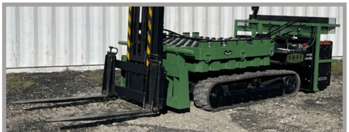
MULE with PA and Fork Riser Mast(FRM) Tested for 3,500+lbs to 6'
