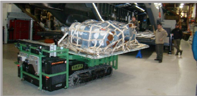
Load/Unload 463L Pallets To/From Cargo Aircraft
