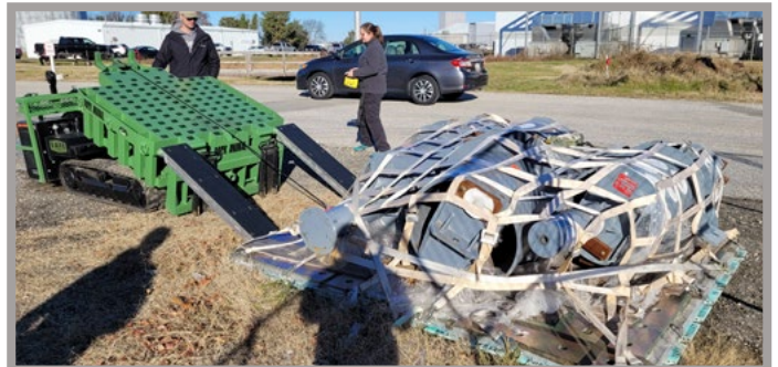
Ability to Load/Unload 463L Fully Loaded From/To Ground
