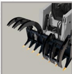
EAGLE TALON - LOG, BRUSH AND ROCK GRAPPLE RAKE
