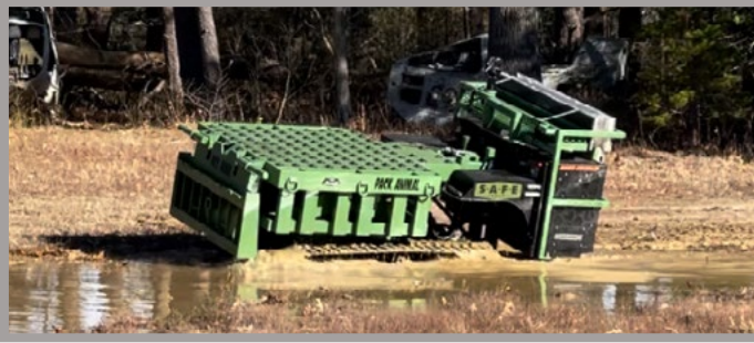
Remote Control Operated with No RF Hard-Wired Cable Option
