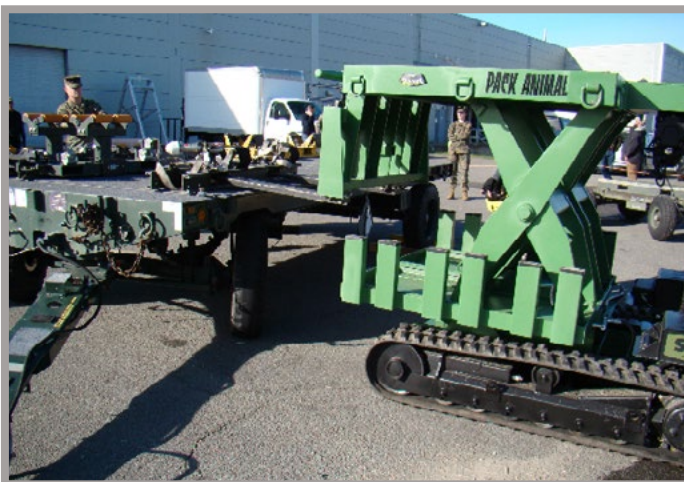
PACK ANIMAL Forks Capable of 4,500+lbs to 36" Height
