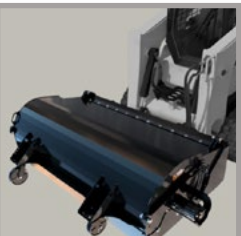
CLEAN SWEEP HD™ - INDUSTRIAL PICK-UP BROOM
