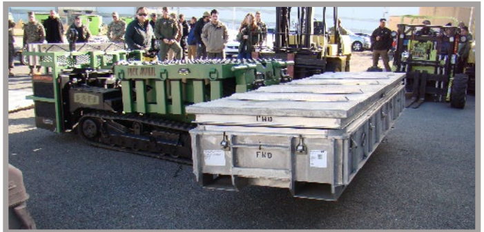
PACK ANIMAL Forks Capable of 4,500+lbs to 36" Height
