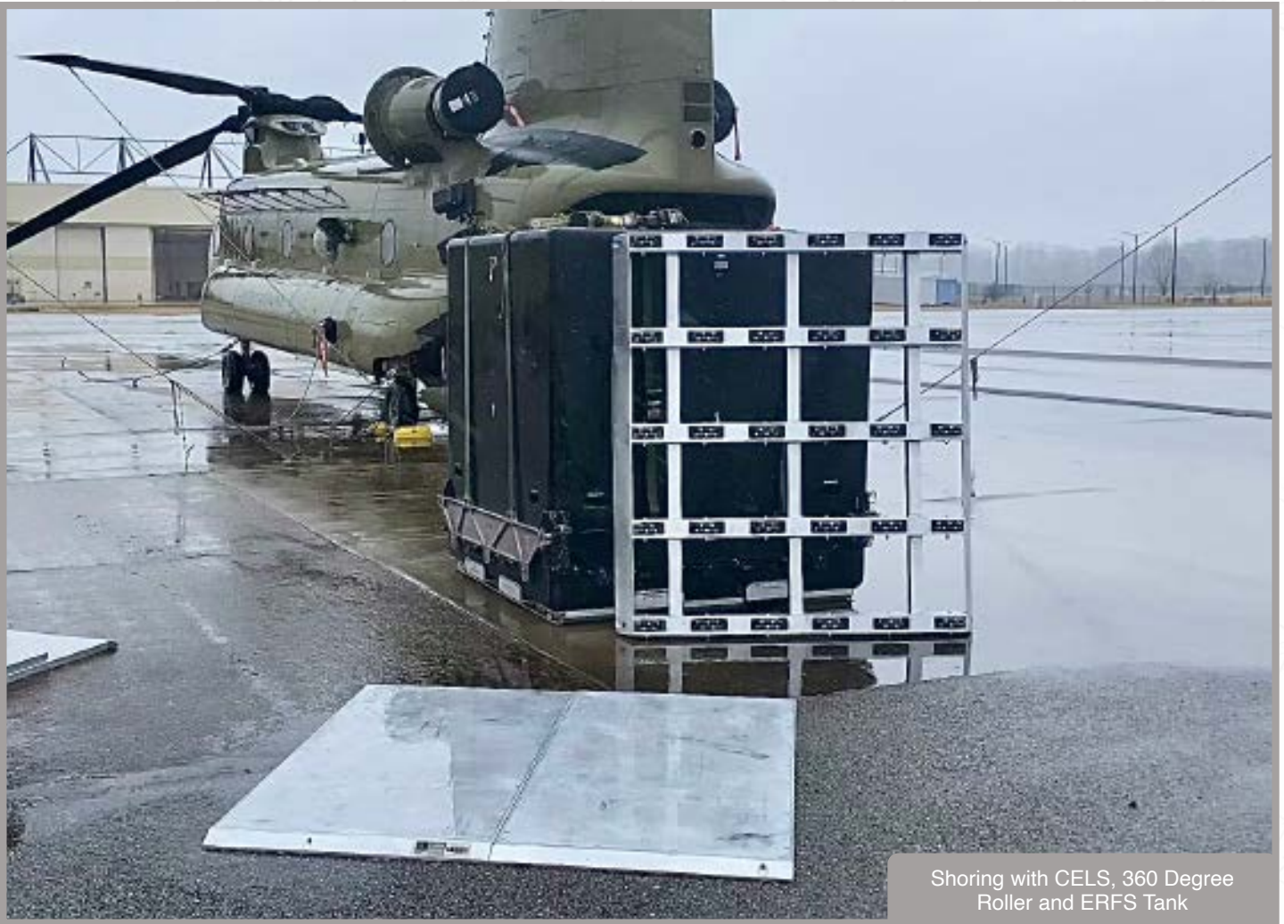
360 Degree Rollers Can Be Towed at Speeds up to a 26 MPH
