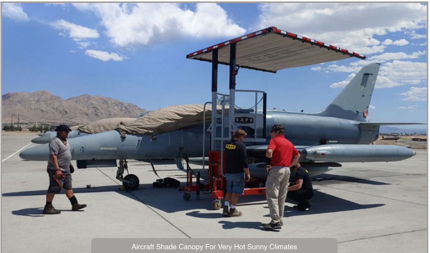
Left Side Stand With Maintenance Stand Dolly For When Aircraft is on a Dolly
